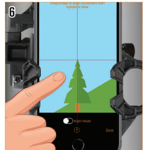
6. Slide the camera view until the same object is centered in the crosshairs.
